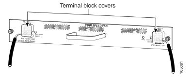
Step 2 The terminal block cover is held in place by two clips inserted into the fan tray front panel. Press the bottom of the terminal block cover, lift the cover up, and remove the cover. (See Figure 12.)
